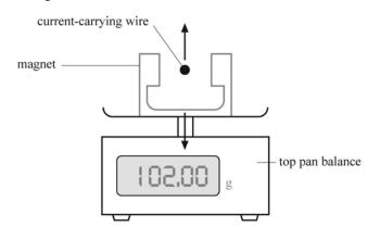
The magnet is placed on a sensitive top pan balance. A current-carrying wire is placed at right angles to the magnetic field between the poles of the magnet. The force experienced by the current-carrying wire is equal but opposite to the force experienced by the magnet. The magnet is pushed downward when the wire experiences an upward force.
